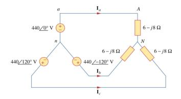
12.13 In the balanced three-phase Y- $\Delta$  system in Fig. 12.46, find the line current  $I_L$  and the average power delivered to the load.
