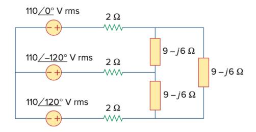
In Fig. 12.56, the rms value of the line voltage is 208 V. Find the average power delivered to the load.
