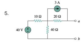
Determine the Thevenin and Norton equivalents at terminals *a-b* of the circuit in Fig. 4.107.
