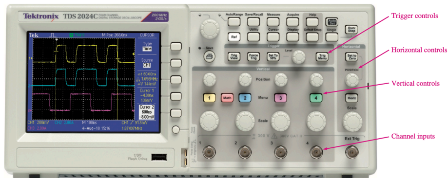
FIGURE 1-44 A typical digital oscilloscope front panel. Numbers below screen indicate the values for each division on the vertical (voltage) and horizontal (time) scales and can be varied using the vertical and horizontal controls on the scope. Used with permission from Tektronix, Inc.
